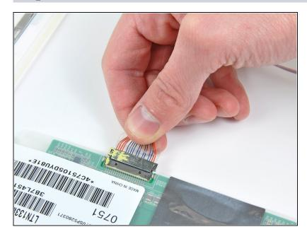
• Disconnect the display data cable from the LCD.
