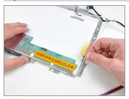
De-route the microphone cable from the clips along the side and top of the LCD assembly.
