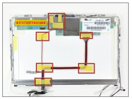
Remove all of the pieces of tape securing your display data cable to the back of the LCD.
