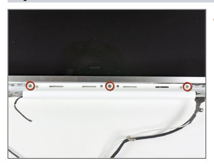
• Remove the three 4.2 mm Phillips screws securing the clutch cover.
