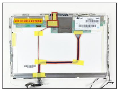
Remove the two pieces of yellow tape covering the camera cable near the top edge of the LCD assembly.
