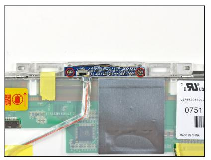
Remove the two 4.1 mm shouldered Phillips screws securing the iSight board to its bracket.
