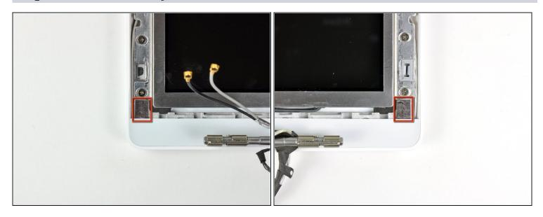
• Remove the small piece of foam tape stuck down above each of the bezel covers, at the lower left and right corners.
