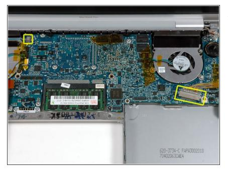
Disconnect the iSight and display data cables from the logic board by sliding the cables out of their connectors, removing tape as necessary.
