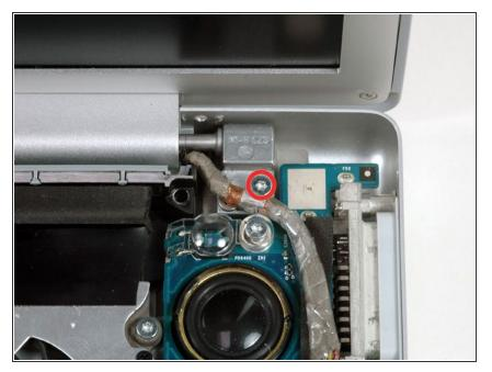
• Remove the silver T6 Torx screw securing the ground loop in the display data cable to the casing.
