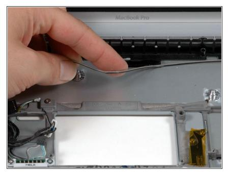
• Continue to free the speaker cable from the black tape until it is free from all three sections of tape.
