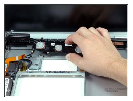
• Lift the heat sink out of the computer.
