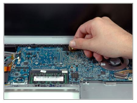
• Peel up the orange Kapton tape securing the right thermal sensor cable to the logic board.
