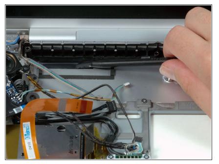
Carefully peel up the black adhesive tape securing the speaker cable along the rear edge of the lower case.
