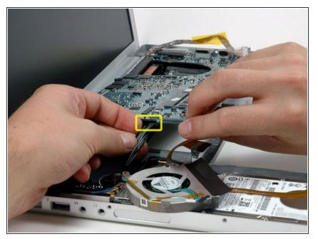
Lift up the left side of the logic board and disconnect the gray and black power cable from the bottom of the board.
