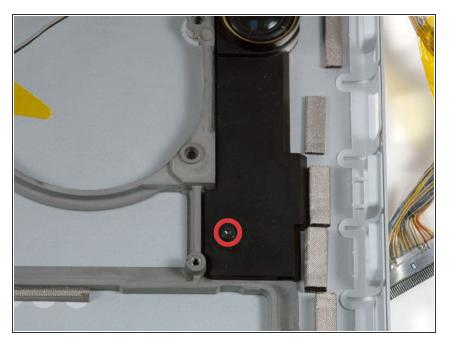
• Remove the single black T6 Torx screw securing the right speaker to the lower case.
