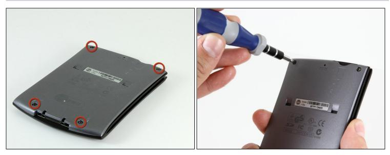
Remove the 4 screws from the corners of the back panel of the device using a size T6 Torx screwdriver.
