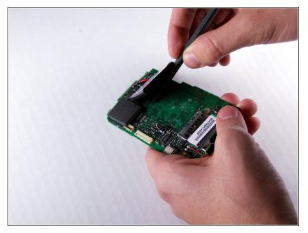
• Using the spudger, pry the battery from where it is glued from the motherboard and observe that the leads are soldered on.
