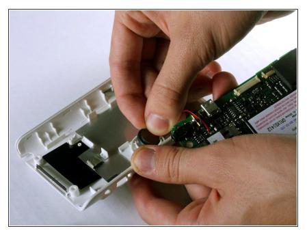
• Carefully remove the speaker from the back white cover by just pulling it gently. It is glued on.
