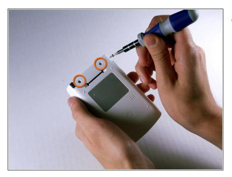
Unscrew the two 7.35mm Torx T6 screws.
