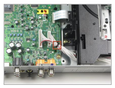
Remove the black tie holding the two rear ribbon cables together by untwisting it.
