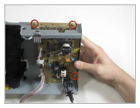
Remove the three .303 inch screws attaching the inverter board to the casing using a #0 Phillips screwdriver.
