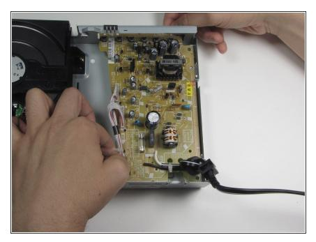
Push the inverter board forward and to the left to remove from the holding ledges.
