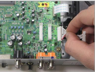
Remove the second of two ribbon cables connected to the motherboard by pulling vertically.
