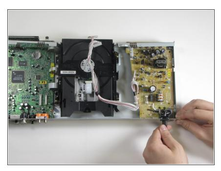
Pull power cord vertically to detach from the casing.
