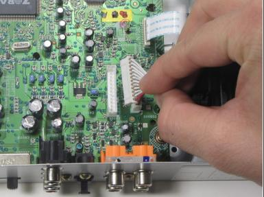
• Remove the first of two ribbon cables connected to the motherboard by pulling vertically.
