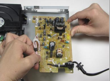
Lift the inverter board from the back end and pull toward you to complete removal.
