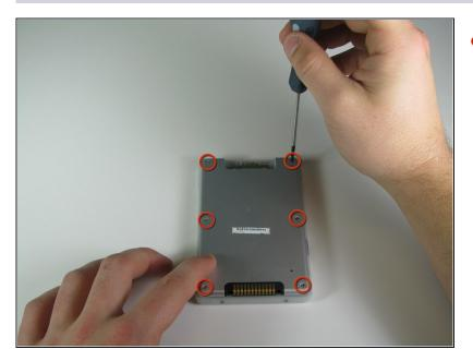
Remove the six 4.1 mm Phillips screws from the back plate using the #00 Phillips Scewdriver.
