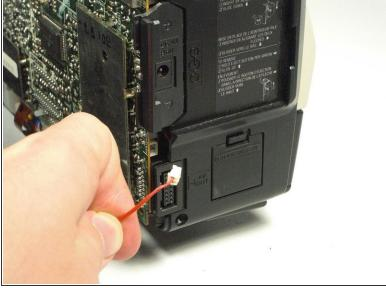
• Unplug the red cable connecting the speaker to the motherboard.
