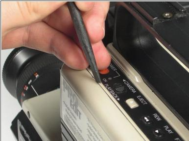
Pry along the seam on the top side near the buttons with a spudger.
