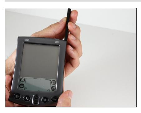
Remove the stylus from the side of the PDA by sliding it upwards.
