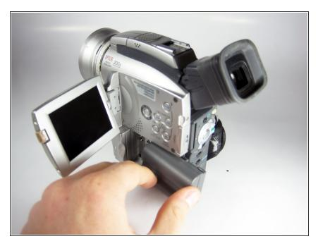
While holding the battery release button to the side, slide the battery towards you, past the release button.
