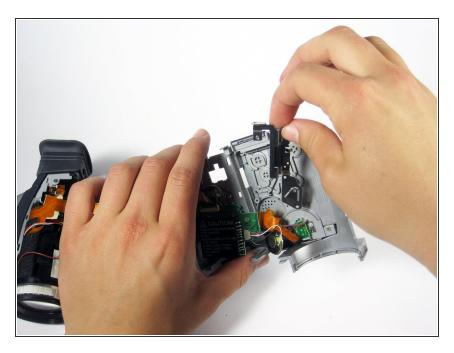
Remove the metal piece partly covering the Button Pad
