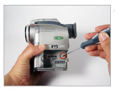
Remove the #00 Philips 4mm screw shown.
