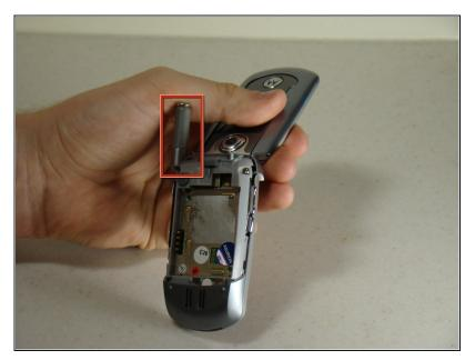
Locate the antenna port on the top of the phone.
