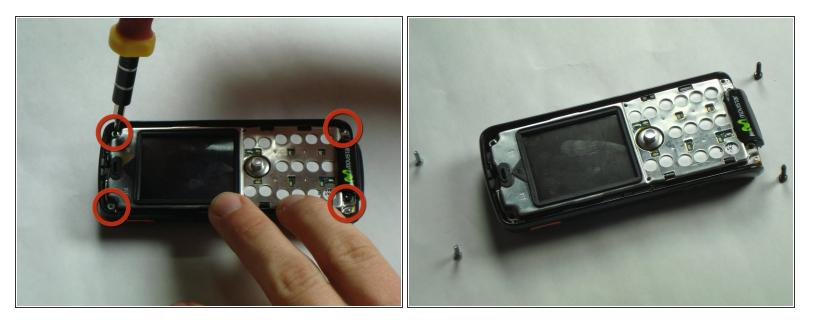
Remove the 4 screws in the corners of the front of the phone using a T6 screwdriver.
