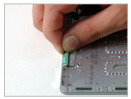
Lift the Bluetooth antenna out of its housing in the upper case. The Bluetooth antenna is secured to the upper case with an adhesive, so rocking the antenna board from side to side may help it come free easier.
