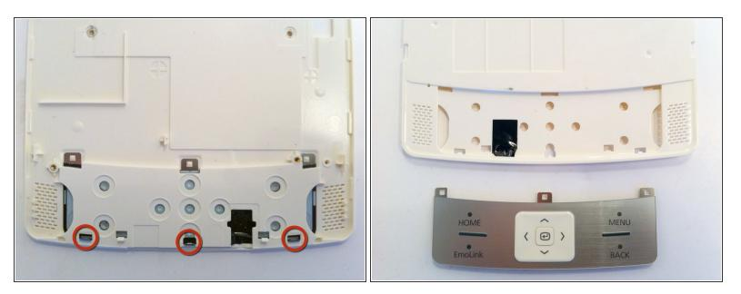
Push in the 3 small metallic hooks from the back of the keyboard to release the brushed aluminium keys
