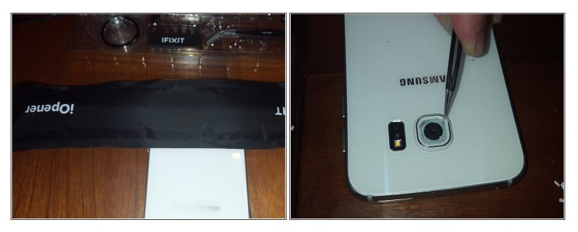
• After clearing all the glass, you will want to remove as much as the old glue as possible. A small set of tweezers like what you get with the iOpener set is perfect. I went ahead and used the iOpener to make the glue a little easier to pull right off.
