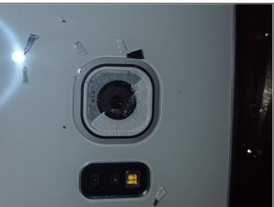
Be careful when removing the shattered glass. You want to make sure the pieces don't fall inside and get trapped next to the camera. You also want to make sure that the lens on the camera itself is not in need of replacement. To do that you would need to remove the back cover and fortunately, I did not have to do this to complete my repair.
