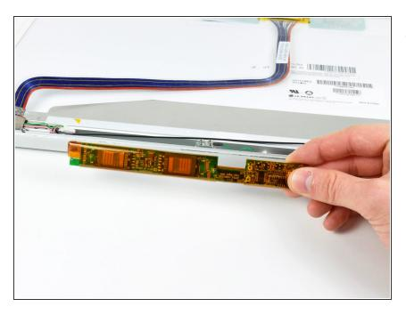
Remove the inverter from the display.
