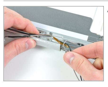
Pull the inverter and antenna cables out of their slot in the clutch hinges.
