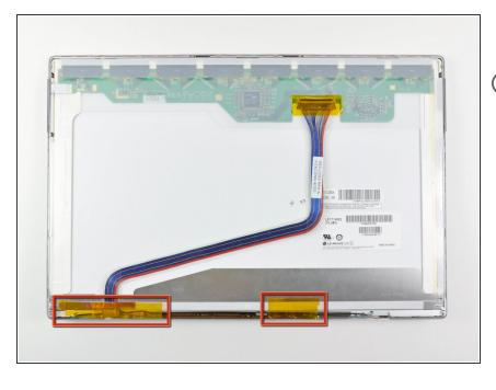
if present, remove the pieces of tape along the bottom edge of the LCD.
