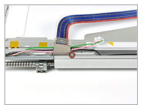
Remove the 2.7 mm Phillips screw securing the display data cable ground loop to the front display bezel.
