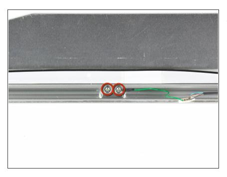
Remove the two 10.3 mm T8 Torx screws securing the center of the clutch hinges.
