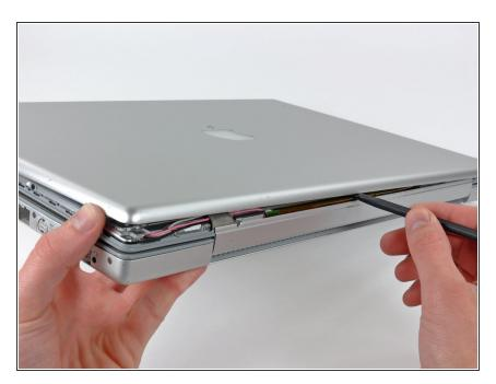
Slightly lift the recently-freed corner of the rear display bezel to separate the clips with a spudger along the span of the clutch hinges.
