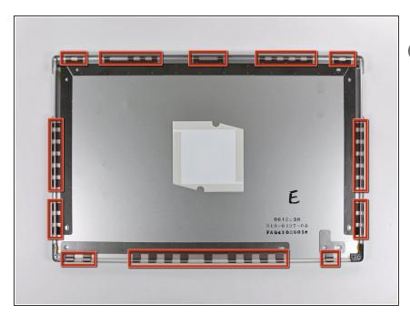
The picture at left (rear panel already removed) shows the locations of the metal clips (shown in red) that snap on to the front display bezel. In the next few steps, you will use a small flathead screwdriver to release these clips from a ridge around the perimeter of the front display bezel.
