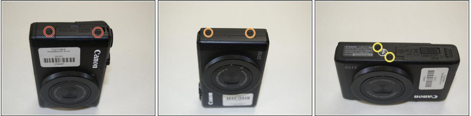
**i** Use a #0 Phillips screwdriver to remove the following screws:
