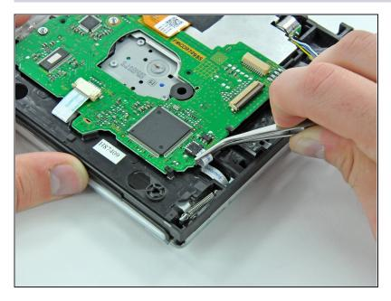
Pull the disc detector ribbon cable straight out of its connector with a pair of <u>tweezers</u>.
