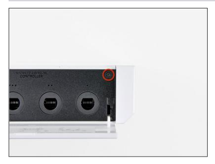
• Remove the single 5.9 mm Phillips screw under the controller port door nearest the faceplate.
