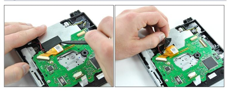
• Remove the piece of black cloth tape that covers a portion of the lens ribbon cable.
