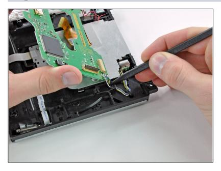
De-route the cables that are soldered to the DVD drive board from underneath their black plastic tabs with the tip of a spudger.
