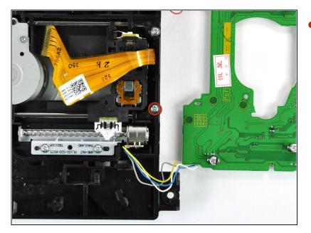
• Remove the 5.0 mm Phillips screw that is closer to the yellow, blue, white, and grey wires.
