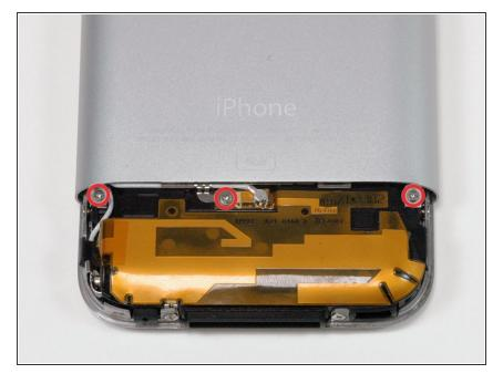
Remove the three Phillips #00 screws securing the rear panel to the iPhone.
