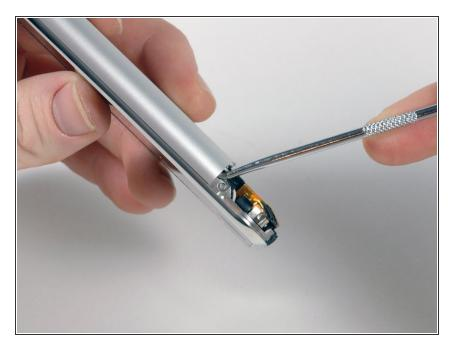
Repeat the same procedure on the other side of the iPhone. Slide the dental pick completely into the square hole. You may need to wiggle the tool and apply a good amount of force to get it to go all the way.
