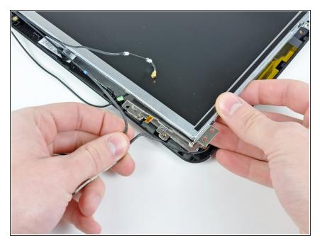
Lift the lower right corner of the LCD enough to de-route the antenna cables from its frame.
