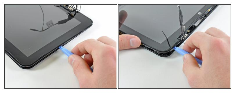
Finally, use a plastic opening tool to release the retaining clips along the left side and bottom left corner of the display.
