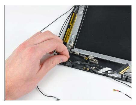
Lift the left edge of the LCD out of the rear display bezel and de-route the cables from the brackets along the left side.
