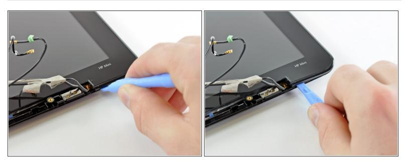
• Use the edge of a plastic opening tool to pry up the front display bezel near the right display hinge.
