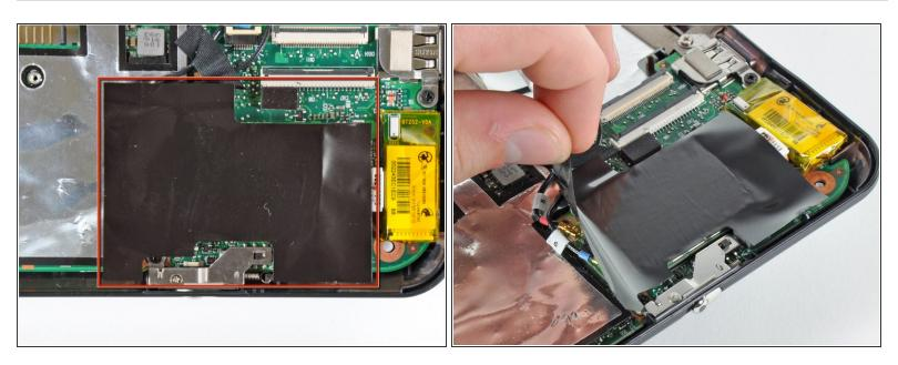
(i) If present, carefully remove the large piece of black adhesive film covering the Wi-Fi board.
