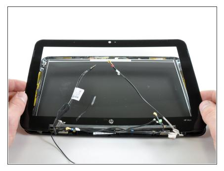
Remove the front display bezel from the rest of the display assembly.
