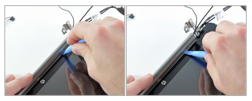
Use the edge of a plastic opening tool to pry the left side of the speaker grill away from the display assembly.
