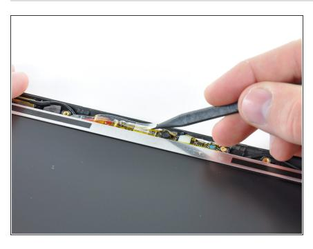
Use the sharp end of a spudger to flip up the plastic flap that rests on top of the camera board cable ZIF socket.
