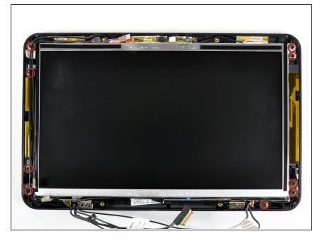
Remove the nine 3 mm Phillips screws securing the LCD to the rear display bezel.
