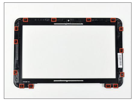
In the following steps you will pry the front display bezel off the rear section of the display. The locations of the retaining clips are highlighted in red.
