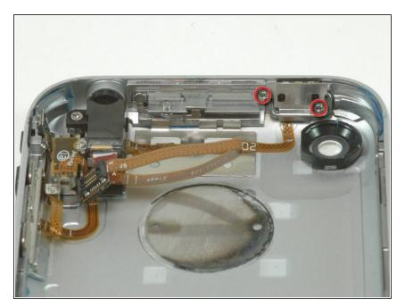
Remove the two Phillips #00 screws securing the on/off switch to the rear panel.
