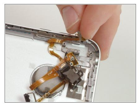
• Grasp the silent/ring switch and lift it up to reveal the screw beneath.
