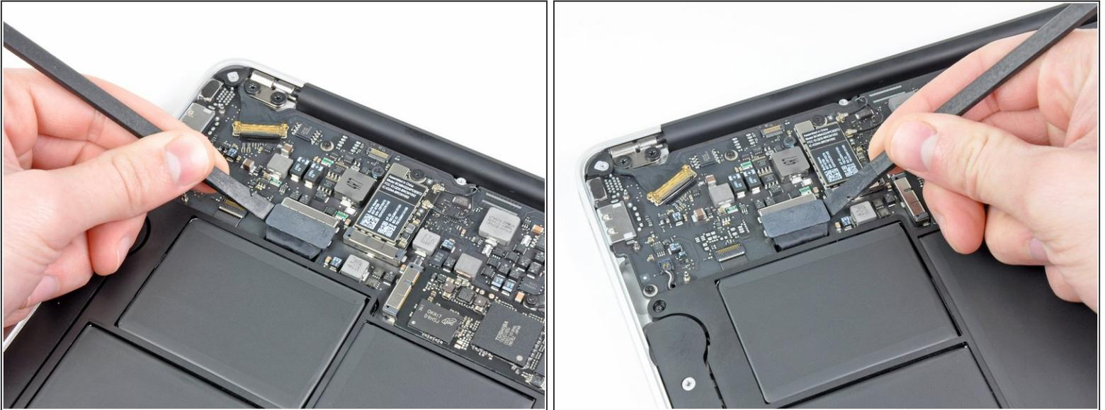
**⚠** In this step you will disconnect the battery to help avoid shorting out any components during service.
