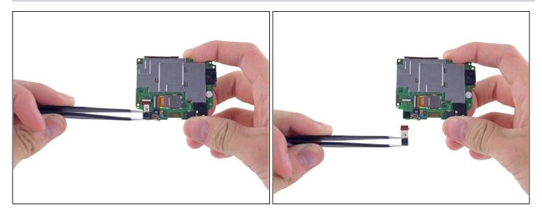
• Gently remove the front camera with a pair of tweezers.
