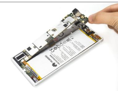
Release flex connectors on the board and remove the motherboard.
