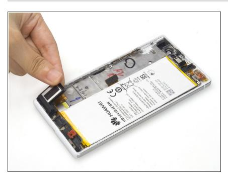
Remove the loudspeaker assembly.
