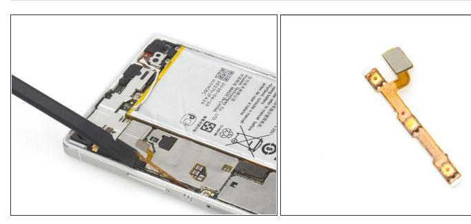
Use the tweezers or some tools thin and sharp to cut the adhesive between power flex and bracket. And then pry it up and remove it.
