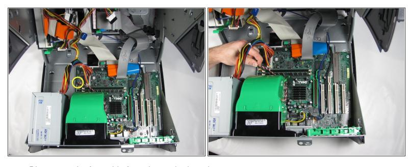
Disconnect the fan cable from the motherboard.
