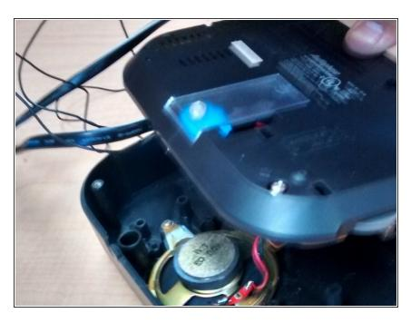
Pull off the bottom casing of the device gently by slowly pushing the bottom part off on all sides of the device. Pull gently on the casing as there are wires that are connected to it still.
