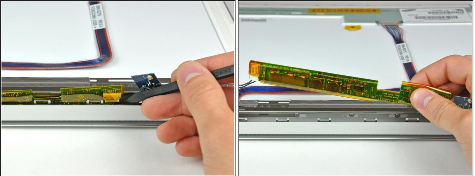
**⚠** The inverter is an extremely thin circuit board that is very delicate and easily cracked. Take care when handling.
