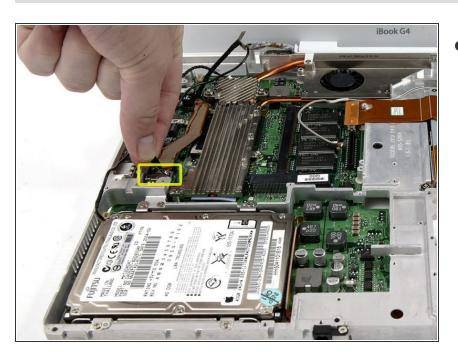
Use the black plastic loop to disconnect the display data cable from the logic board.
