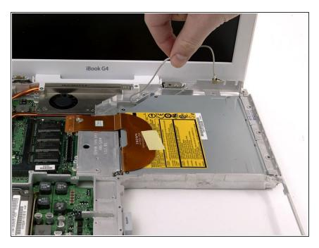
Deroute the AirPort antenna cable from the metal framework, removing tape as necessary.
