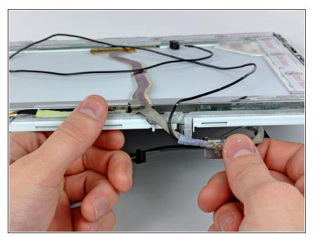
Remove the display data cable from the display. To reassemble your device, follow these instructions in reverse order.
