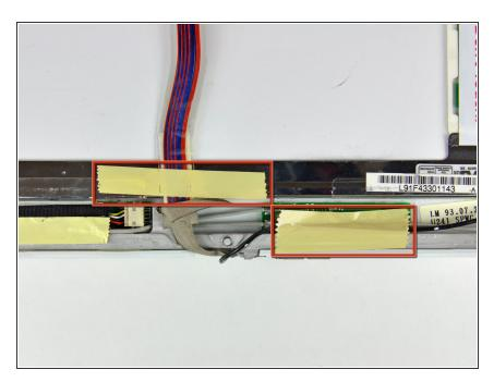
Remove the pieces of tape covering the display data and microphone cables near the bottom edge of the display.
