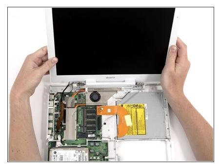
Lift the display up and tilt it backwards, freeing it from the two metal alignment posts holding the hinges in place, and slide it away from you.
