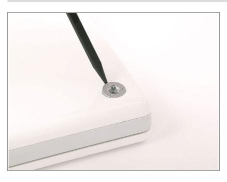
Use a spudger or small flathead screwdriver to pry up the three metal rings that housed the rubber bumpers.
