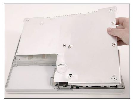
Lift the bottom shield off.
