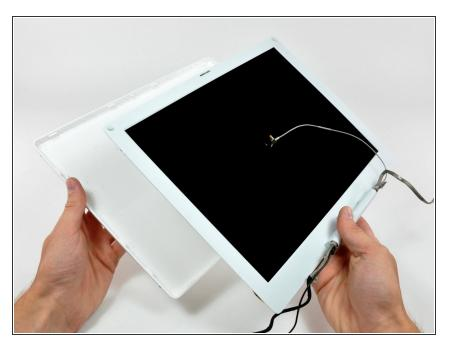
Lift the rear bezel off the display.
