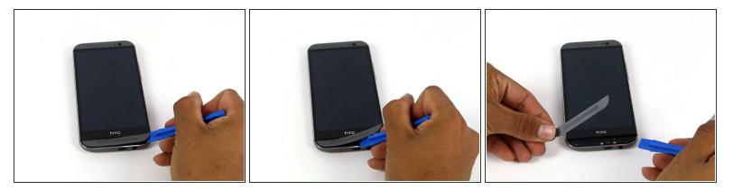
• Use a plastic opening tool to gently peel up the lower speaker grille.
