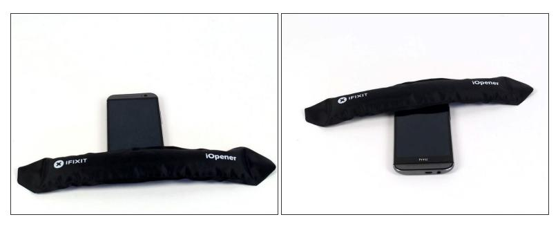
Use an iOpener or heat gun to loosen the adhesive on the upper and lower speaker grilles.
