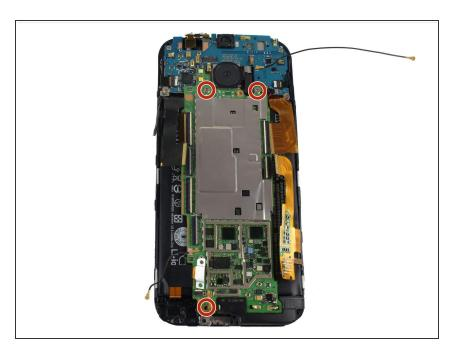
Remove three silver 3mm screws using T5 screwdriver.
