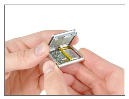
Remove the rear panel from the Shuffle.
