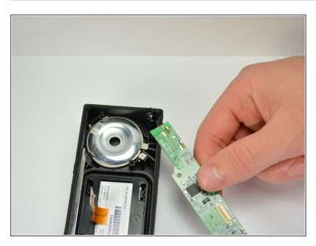
Carefully lift the motherboard out of the plastic housing.
