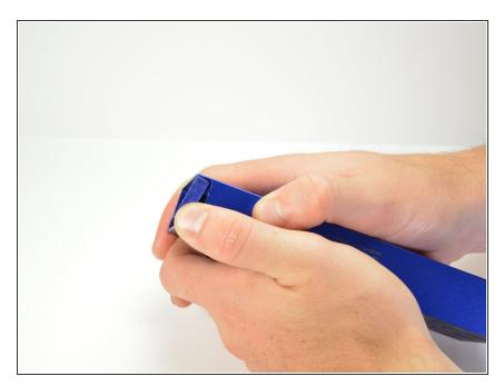
Slide out the rubber foot located on the bottom of the case.
