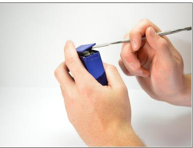
Using the standard metal spudger, begin by prying at the bottom of the plain rubber end cap (the end without the USB or auxiliary input).
