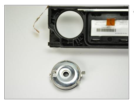
Replace the blown speaker with a new one and reassemble the JAMBOX.
