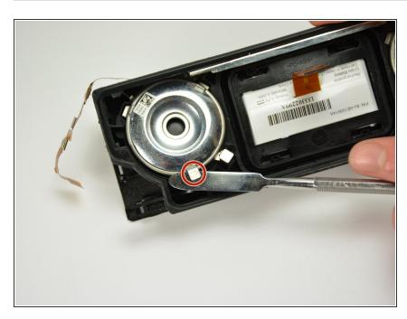
Carefully lift the speaker out of the plastic casing using the rotated metal tabs.
