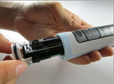
Push the flat edge of a nylon or metal spudger between the seal and the toothbrush body and pry it up. Do this on each side until the seal is partially sticking out on all sides.
