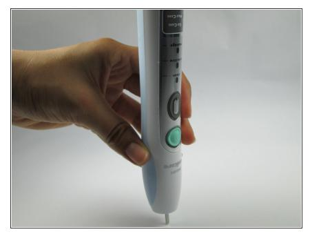
Apply pressure to the shaft by pressing it against a firm and flat surface. Continue to apply pressure until the interior electronics are exposed.
