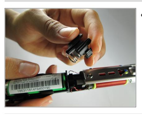
Remove the spring from the rubber ring and replace it with the new spring.
