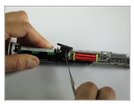
Pull off the black rubber ring with a metal or nylon spudger until it clears the metal piece that holds it in place.
