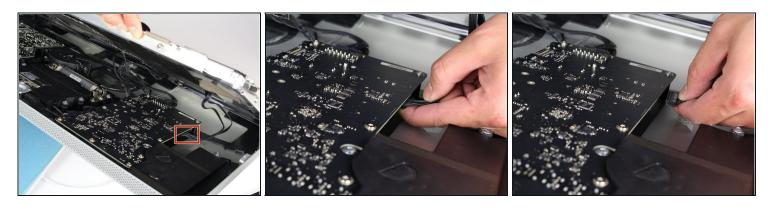
• For the connector on the other side of the logic board, grab the connector from underneath and carefully pull it from the board.
