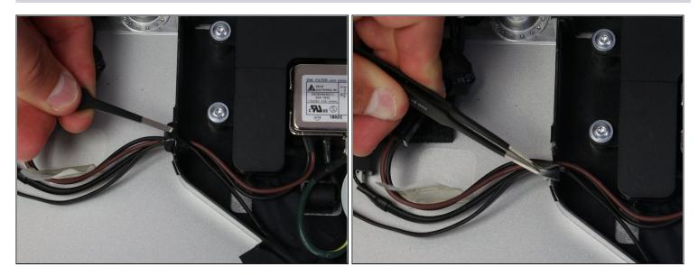
• Next, remove the piece of electrical tape that is holding wires into the casing connecting to the power adapter.
