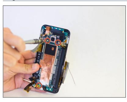
• Remove the three 4 mm T5 Torx screws that secure the motherboard.
