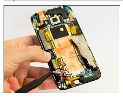
Use a pair of tweezers to get underneath the white and blue cable connectors and gently push them upwards to disconnect them.
