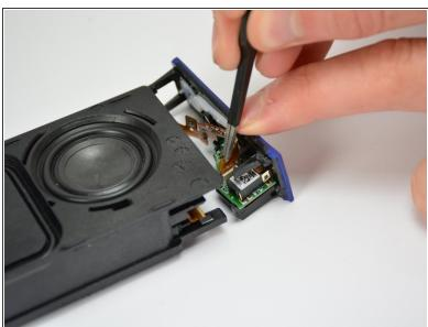
Reconnect the button ribbon connector on the top of the port assembly.
