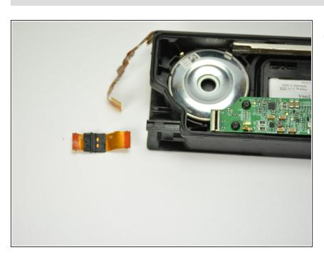
Very carefully pull the motherboard connection ribbon through the plastic casing, removing it from the plastic casing.
