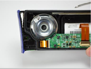
Using the standard metal spudger, carefully pry up the top 2 plastic tabs which hold the exterior button and port cover onto the interior plastic frame.
