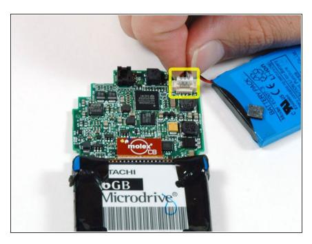
Carefully disconnect the battery from the logic board. Make sure to pull only on the connector and not on the battery wires.
