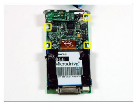
Note the location of the four white plastic tabs securing the display to the logic board. These tabs must be released before the display can be removed.
