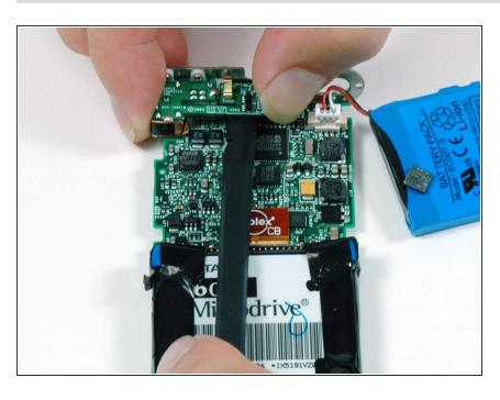
Use a spudger to carefully pry up the headphone jack board from the logic board. Be careful to pry up
