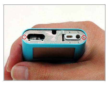
Remove the two #00 Phillips screws securing the headphone jack to the casing.
