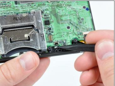
• Use your fingernail or the edge of a plastic opening tool to carefully flip up the touchscreen ribbon cable retaining flap.
