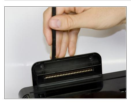
Using the spudger, pry the cover off of the Genesis attachment.
