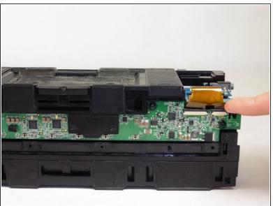
Remove the colored ribbon that connects the green button circuit board to the blue auxiliary board by using your finger to lift the small black tabs that clamp down the ribbon.
