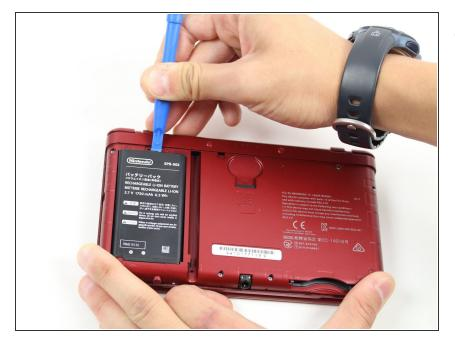
The battery is located on the left hand side of the 3DS - to remove, use the small gap located at the topmiddle and pull up with a non metal pointed tool.
