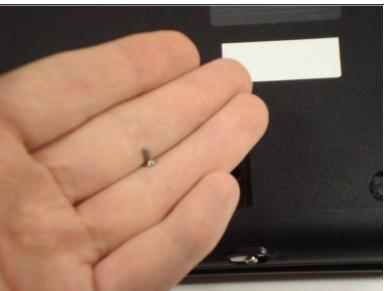
Unscrew the screw for the bottom case located in the RAM compartment.
