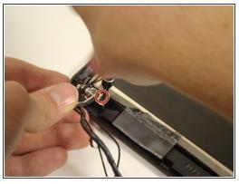
Remove the 4 screws keeping the screen on the plastic assembly.
