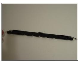
Unscrew the speaker assembly at the bottom of the screen assembly.
