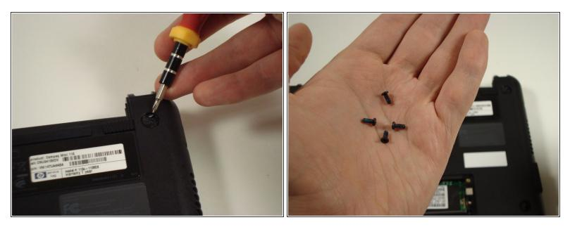
• Unscrew all the corner screws. There are four total, one under each rubber pad.
