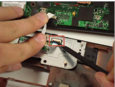
Remove the cable by carefully pulling it up.
