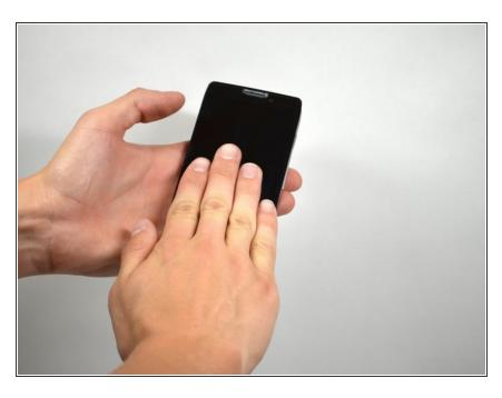
Holding the device in your hand, push the screen towards the top of the phone until it disconnects from the base of the phone.
