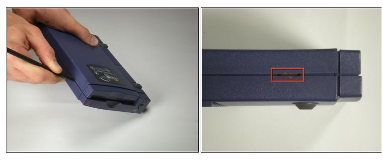
• Push in the plastic tab that can be seen through cracks in the front left corner using a spudger.
