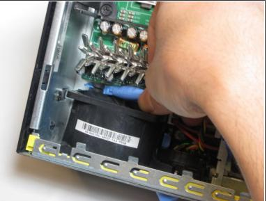
Remove the rubber grommets from the base of the fan. A spudger may be useful.
