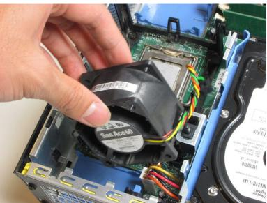
Press on the blue release tab and remove the fan.
