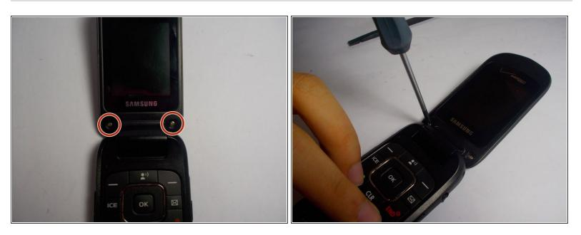
• Remove the two screws near the front screen.
