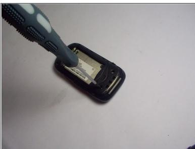
Remove the four screws shown using a small screwdriver.
