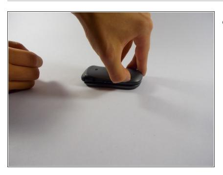
Place the phone down flat and remove the back panel as shown.
