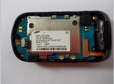
• Use a prying tool to remove the back cover of the phone. Once part of the cover is popped off, run the tool along the length of the edge to remove the cover.
